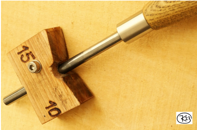
Figure 28: Another guide (10° and 15°, e.g. for smaller specially shaped card scrapers)
