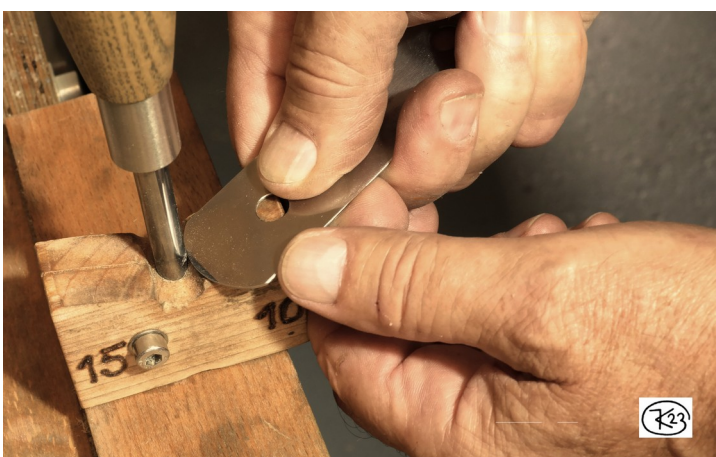
Figure 23: Forming the cutting burr on a small scraper with a convex edge.
