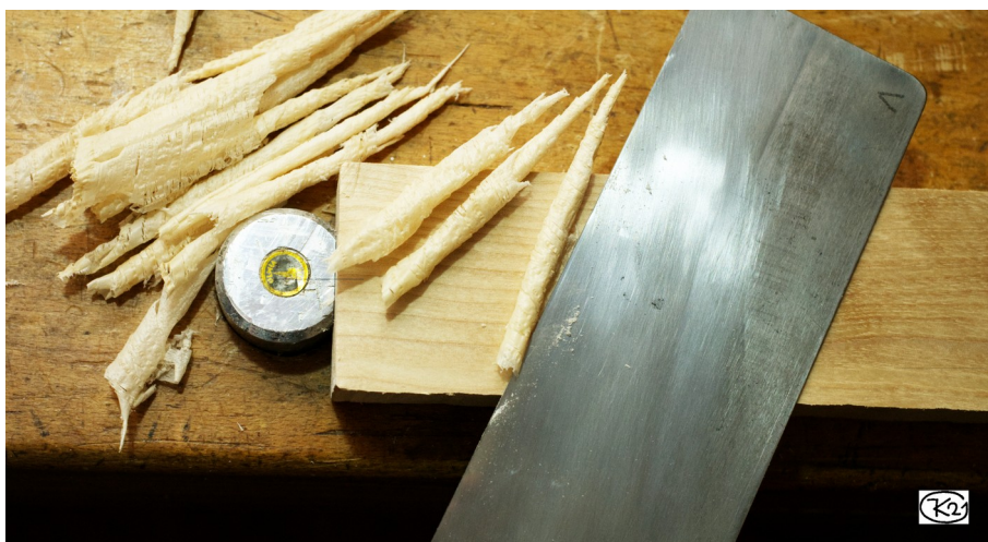
Figure 18: Shavings from a well sharpened card scraper
