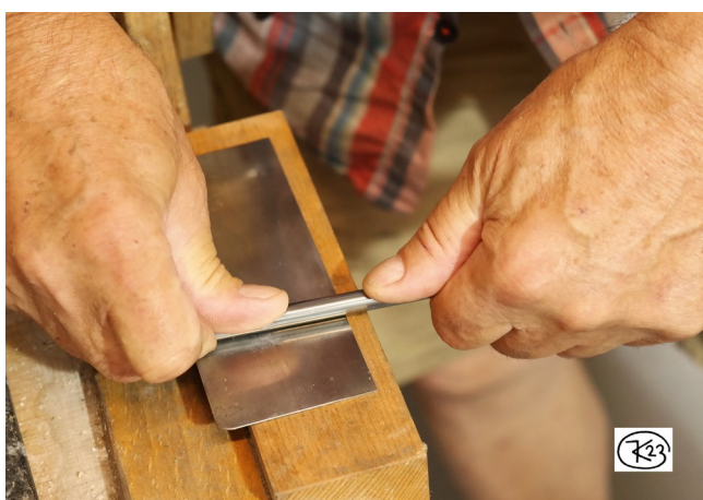
Figure 19: pushing back a dull cutting burr as the first step to refresh it (card scraper rests on a piece of hard-wood).
