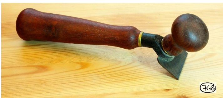
Figure 3: Scraper with handle (Veritas)
