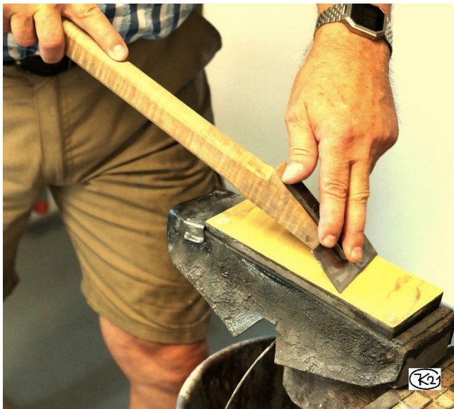
Figure 24: Free hand grinding of a 45° scraper blade with a holder
