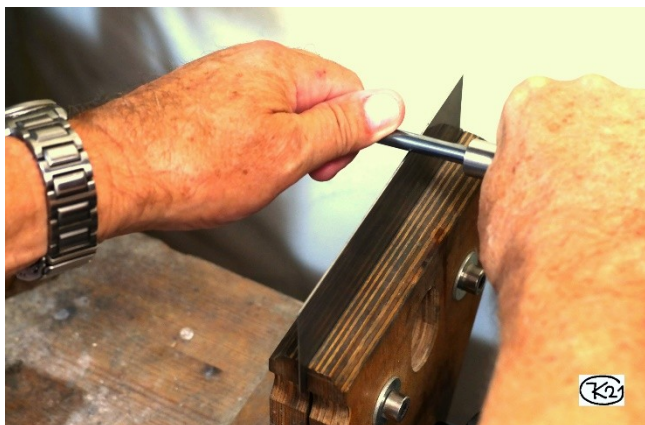
Figure 17: Forming the cutting burr
