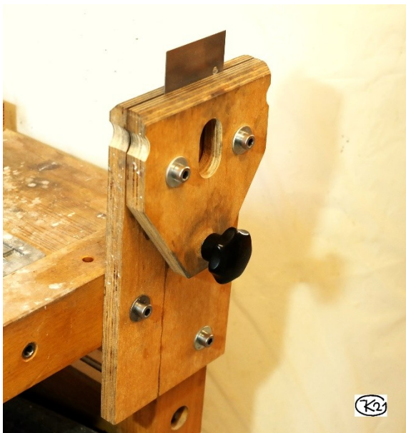
Figure 31: Vise for card scrapers
