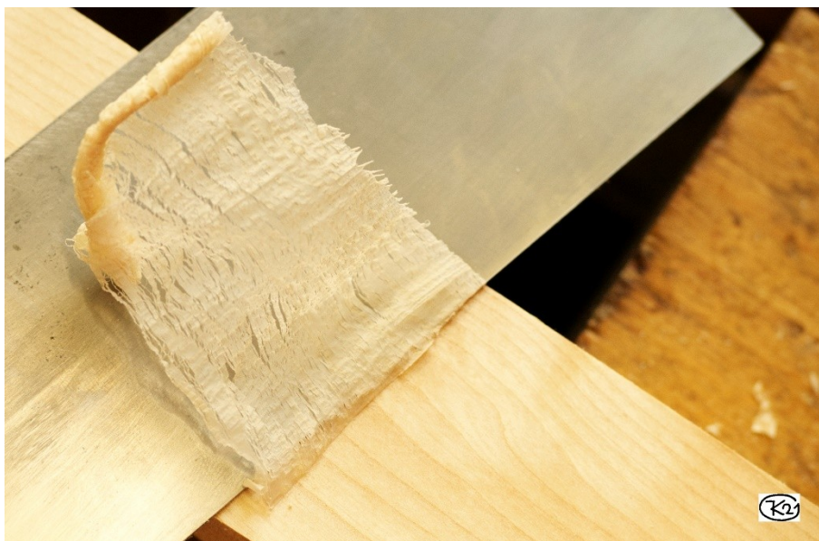
Figure 21: Shaving from an extensively prepared 90° card scraper
