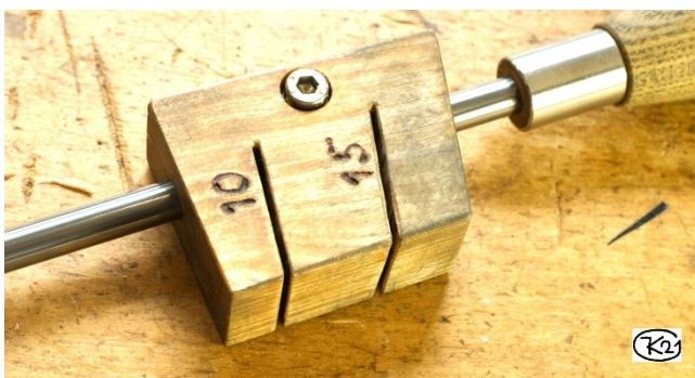
Figure 27: 10° / 15° guide with slots
