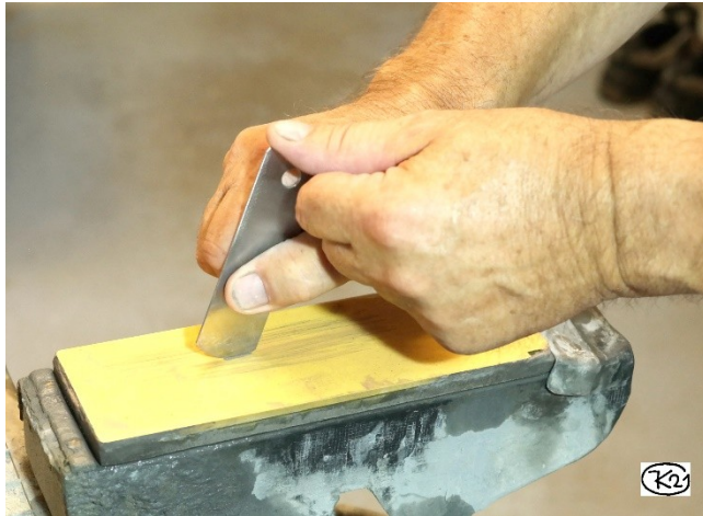
Figure 22: free hand grinding of a convex edge face (Example)
