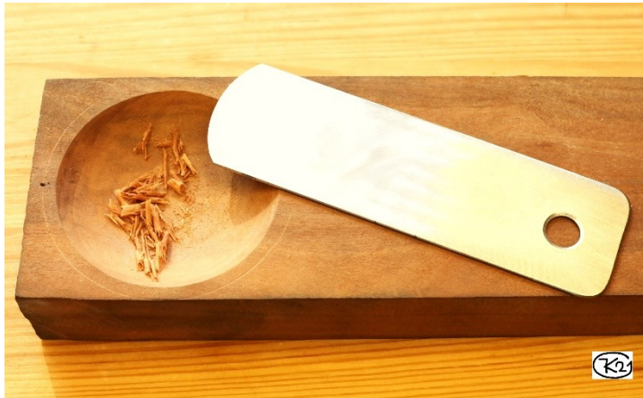
Figure 34: Bowl of a cooking spoon, smoothed with a card scraper
